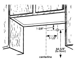
**To wire through rear,** mark a line 7-1/2" from the right of the centerline on the wall. Mark the point on this line that is 64-5/8" from the floor (or 1-3/8" from underside of cabinet). Drill a 1-1/4" diameter hole through wall at this point.
